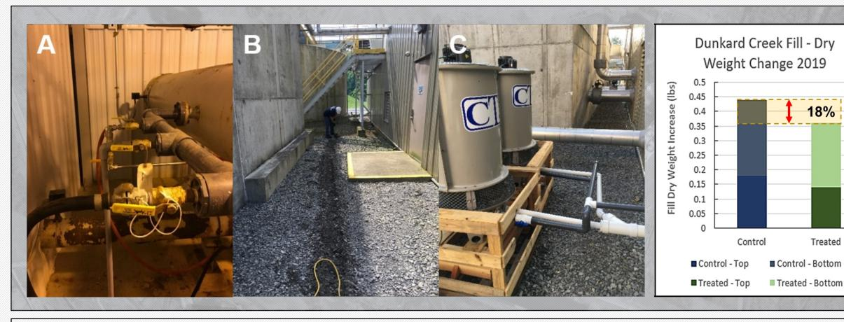
THERMOPHASE treatment reduced dry weight by 18%. Small-scale cooling towers installed at water treatment station, circulating raw untreated water over the 2019 fouling season. Towers treated with Interphase technology showed increased fouling resistance, accumulating 18% less dry weight fouling.
