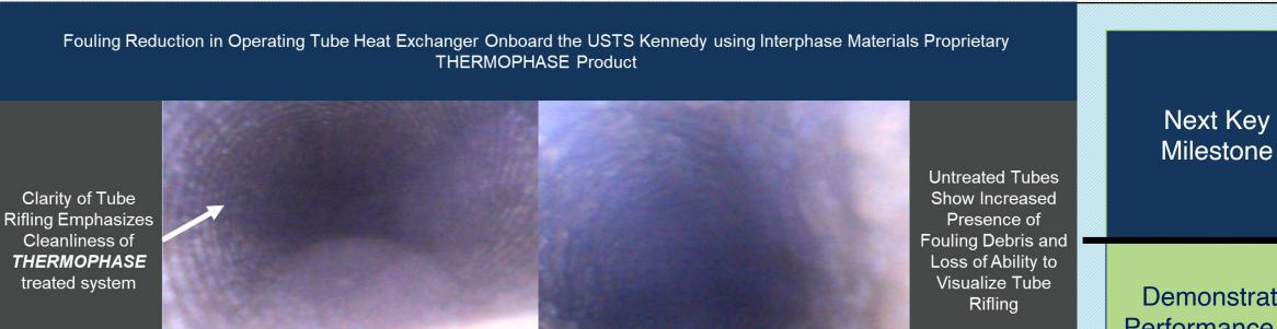
This demonstration occurred using a 1 hr flush of THERMOPHASE product on the USTS Kennedy's HVAC chillers. These chillers are fed raw seawater without treatment. The duration of this demonstration 4 months based on the ships schedule. A reduction in fouling observed here will provide significant benefits to the operation of the system and in costs/time associated with system maintenance.
