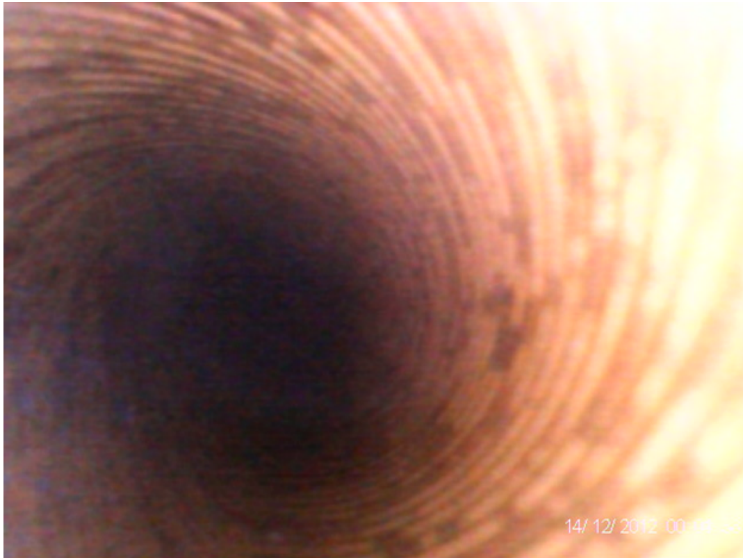
Image 2: Borescope Image of Chiller Tube After Cleaning from UPMC Children's Hospital Chiller in 2021
